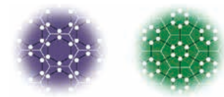
Schematic cross-sections of the two types of crystals used to generate laser radiation Topological photonic crystal (left) and matching non-topological photonic crystal (right). Wrapping the crystal on the left with the crystal on the right forms an optical resonator required for a laser.
