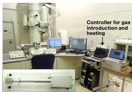
The TEM system The complete TEM system assembly being used for observational study and the newly developed specimen holder (lower left)
