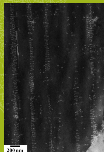
SEM-ECC image of dislocation pile-ups in a 316 L stainless steel
