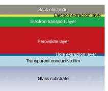
Figure 2 : Structure of a perovskite solar cell.
