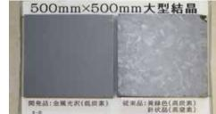
Figure 2 : Mono-crystal silicon created using the single-seed cast method (left). Unlike the conventional product (right), the new product has a metal-like smooth and shinv surface
