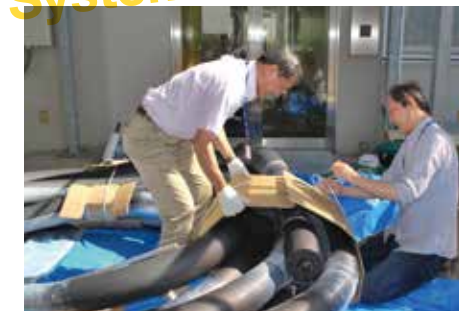
Making a simple insulated pipe for transporting liquid nitrogen
