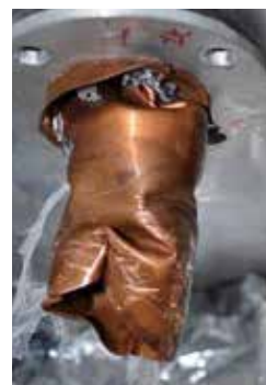
Room temperature bore magnet tube (copper tube of 56mm diameter and 4m long) 10 ton weight shaken by horizontal oscillation of earthquake caused the vacuum break.
