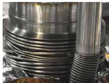
Bellows broken by the earthquake
