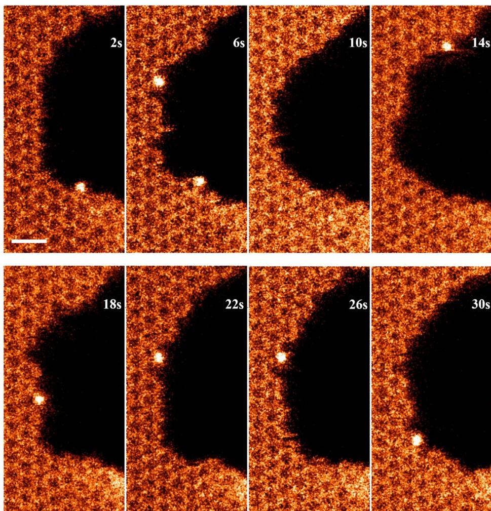
**Fig. 3.** Time sequence of ADF images showing the modification of a graphene edge and the diffusion of Si adatoms under 60 kV electron beam illumination. In the second frame, the Si atom was captured twice during the acquisition of the STEM-ADF image as it migrated from the top to the bottom along the graphene edge. Scale bar: 0.5 nm. Frame time: 2 s.
