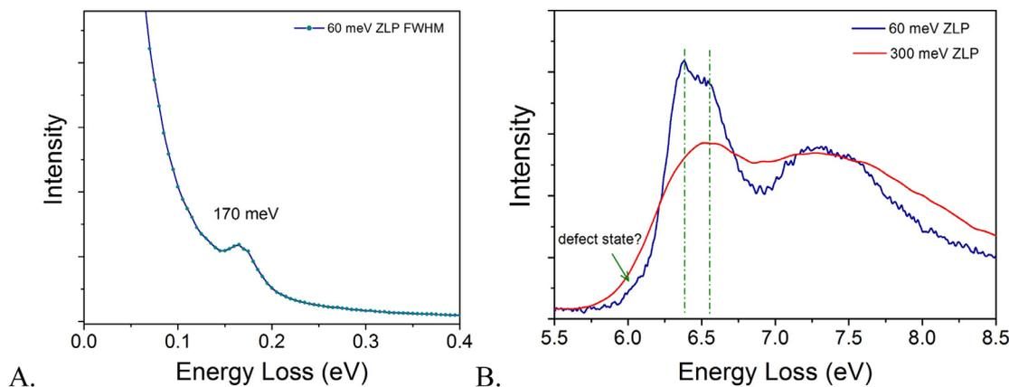
**Fig. 5.** Monochromated low-loss EELS from thin h-BN flakes (1–2 layers) showing the longitudinal optical (LO) phonon peak (A) and the plasmon peaks (B). The plasmon spectrum is also compared with a spectrum acquired without a monochromator (red curve).
