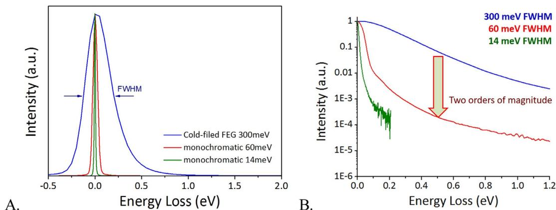
**Fig. 4.** Comparison of the ZLP from a CFEG with and without a monochromator. The resolving power at the low energy loss regime, especially below 1 eV, has been drastically improved by the monochromator. (A) ZLP plotted in linear scale showing the changes in FWHM. (B) ZLP plotted in log scale to highlight the suppression of the intensity at the ZLP tail.
