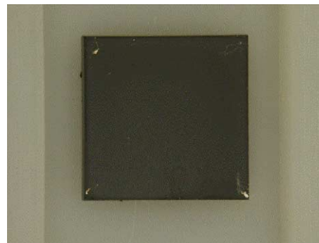
Fig. 1. Optical microscopy image of the polycrystalline diamond thin film deposited by MPCVD method.
