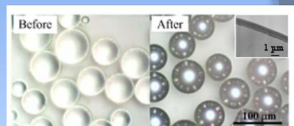
**Figure 1** Optical microscope images of PMMA particles (particle size: 50  $\mu\text{m}$ ) before and after Pt sputtering. Inset shows the cross-sectional TEM image of a Pt-sputtered particle [1].
