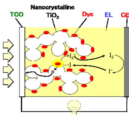
Fig.1 Schematic of dye-sensitized solar cells.
