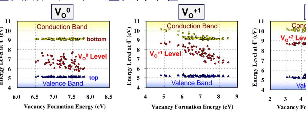
Vacancy formation energy:  $H_f = E_{\text{defect}}^q - E_{\text{perfect}} - n_{\text{O}} \mu_{\text{O}} + q(\epsilon_{\text{F}} + E_{\text{VBM}})$ :  $n_{\text{O}} = 1, \epsilon_{\text{F}} = \frac{\epsilon_{\text{g}}}{2}$
