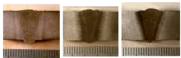
(a)パルス電流制御 (b)位相制御 =0.72 (rad) (c)位相制御 =1.4 (rad)
