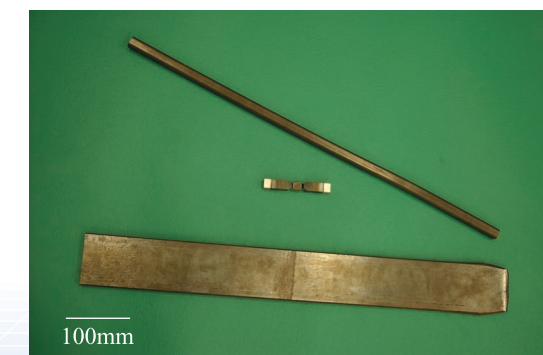
Double strength steel (Top) Steel bar 18 mm square (Middle) Specimen formed by multidirectional deformation method (Bottom) 16mm thick plate
