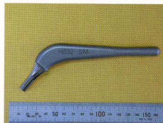
A stem for an artificial hip joint (Length:150mm)
