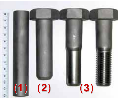
Fig.10 Forming process of ultra-high strength steel bolts by prototype steel (1800MPa steel)
