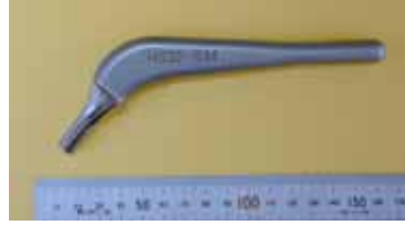
Fig. 6 Example of hip-joint stem made by Ni-free HNS
