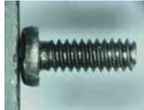
Fig. 3 Screw manufactured from ultra fine grained steel (M1.6)
