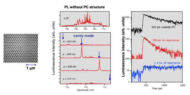
(Left) SEM image of a photonic crystal micro cavity embedded with GaAs quantum dots, (middle) shift of resonance wavelength as a function of the lattice constant, a, and (right) suppression and acceleration of spontaneous emission. T. Kuroda et al., Appl. Phys. Lett. **93**, 111103 (2008).
