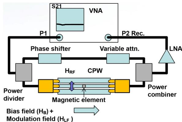
Fig. 1, Block diagram of the I-FMR apparatus
