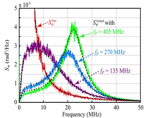
Fig. 2, PESD of the STO output signal. The four lines drawn with red, purple, blue and green represent the PESD when the STO is free running, phase locked to three different reference frequencies of  $f_r = 135$  MHz, 270 MHz and 405 MHz, respectively. The broken line superimposed on each line is the theoretically calculated PESD.
