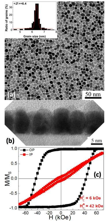
Fig. 1 In-plane and cross sectional TEM image of an optimized FePt-C film deposited by the compositionally graded process.
