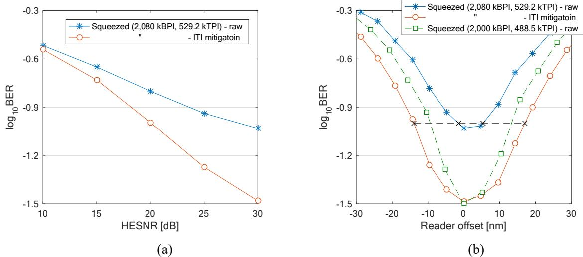
Fig. 2 BER performance of the IMR with the proposed ITI mitigating scheme (a) as a function of HESNR at on-track location with 529.2 kTPI,  $L_s = 2,080$  and  $L_n = 2,600$  kBPI, and (b) bathtub curves at HESNR=30dB with the previous condition, and with 488.5 kTPI,  $L_s = 2,000$  and  $L_n = 2,500$  kBPI for comparison.
