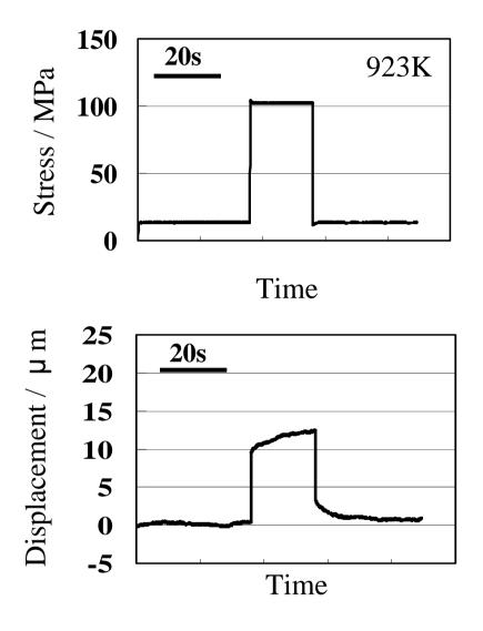
Deformation behavior of the P92 steel upon abrupt stress loading at 923K. Applied stress is 100 MPa.
