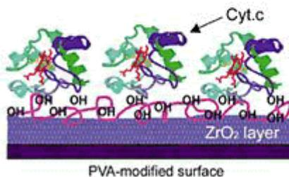
**Schematic illustration of cytochrome c on a metal surface modified with nanometer-thick  $ZrO_2$  and PVA layers.**
