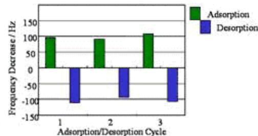
**QCM frequency changes during repeated adsorption and desorption of cytochrome c. The protein completely desorbs in alkaline solution.**
