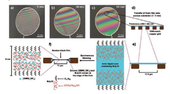
Preparation of Newton black films of Brij-35 using 1-ethyl-3-methylimidazolium tetrafluoroborate
