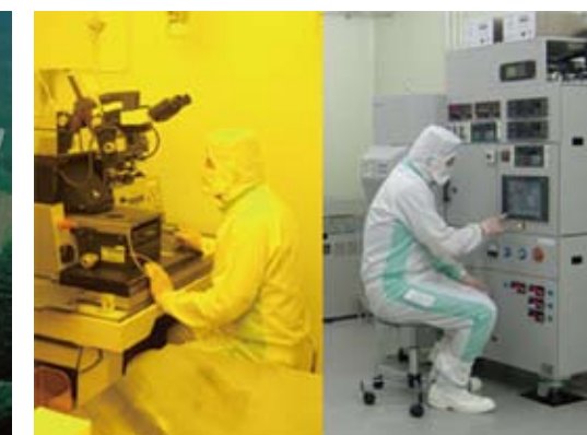
MANA Foundry Both sides mask aligner (left), Sputtering machine (right)
