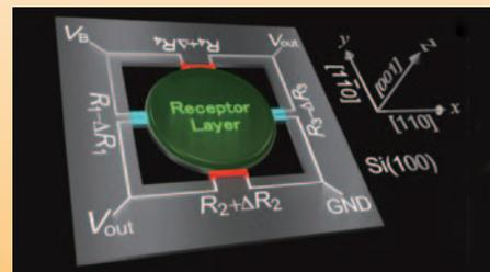
Figure 2. Newly developed Membrane-type Surface stress Sensor (MSS). The surface stress induced by an adsorption of analytes on the center membrane is efficiently detected by the piezoresistors embedded at the four peripheral beams.
