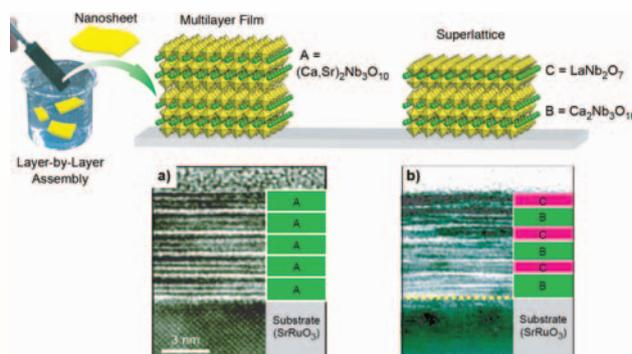
Figure 1. Solution-based bottom-up assembly using oxide nanosheets. Cross-sectional TEM images of multilayer  $(\text{Ca}_{2-x}\text{Sr}_x\text{Nb}_3\text{O}_{10})$  film (a) and  $(\text{Ca}_2\text{Nb}_3\text{O}_{10}/\text{LaNb}_2\text{O}_7)$  superlattice (b).
