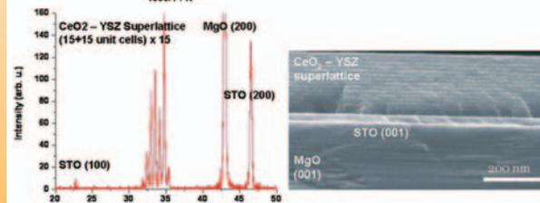
Figure 2. XRD pattern and SEM cross sectional micrograph of a  $\text{CeO}_2$ -YSZ heterostructure grown (001) epitaxially oriented with the  $\text{MgO}$  substrate by means of a thin buffer layer of  $\text{SrTiO}_3$  (STO).
