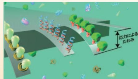
Figure 1. Schematic image of the measurement of various analytes ranging from gaseous to biological molecules using an array of microcantilevers. The deflection induced by an adsorption of analyte molecules is measured as a signal.
