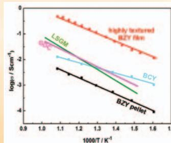
Figure 1. Comparison between the electrical conductivity values of the highly textured films of Y-doped barium zirconate (BZY), and of BZY and BCY (Y-doped barium cerate) sintered pellets, measured in the intermediate temperature range. Conductivity values of the best-performing oxygen-ion-conducting materials,  $\text{La}_{0.8}\text{Sr}_{0.2}\text{Ga}_{0.8}\text{Mg}_{0.2}\text{O}_3$  (LSGM) and  $\text{Ce}_{0.8}\text{Gd}_{0.2}\text{O}_{1.9-\delta}$  (GDC), are also reported.
