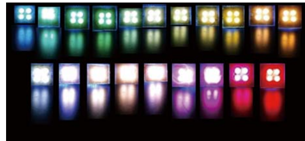
Fig.2 Multicolor light emitting devices prepared by laminating yellow green and red SiAlON phosphors. The electrophoretic deposition process enables easy emission color tuning by controlling the thickness of each phosphor layer.
