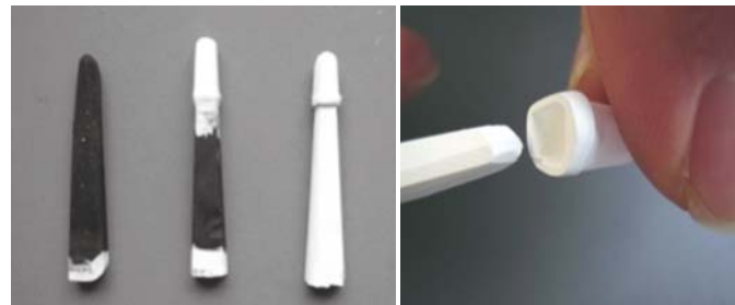
Fig.1 Example in direct shaping of ceramics by electrophoretic deposition using conductive polymer-coated non-conductive ceramic substrates. This technique can be utilized for fabricating various shape-controlled ceramics, such as dental crown.
