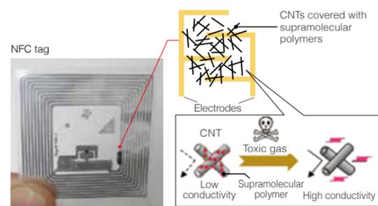
■ Toxic gas sensor embedded in an NFC circuit
