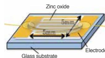
■ Structure of an alcohol sensor
