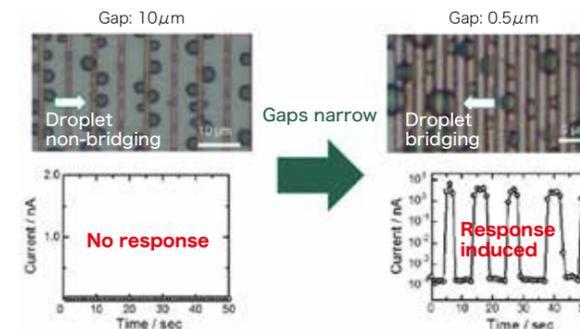
Schematics showing that when water droplets bridge gaps between two adjacent electrodes arranged in parallel, electric current is produced. By using another chip with different electrode gap widths and checking the chips' electrical responses to droplets, the size of water droplets can be determined.
