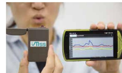
An image of mobile sensor system based on the MSS technology to detect breath components and to monitor health conditions
