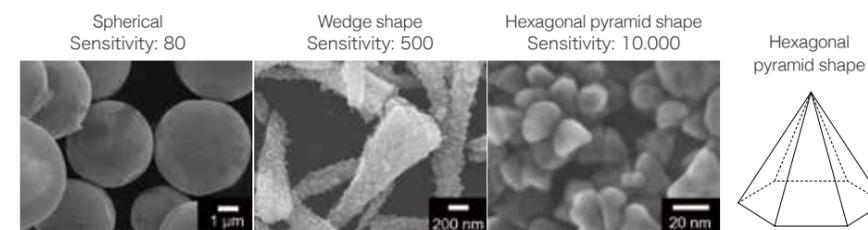
■ Various forms of zinc oxide nanoparticles and their sensitivity to alcohol
