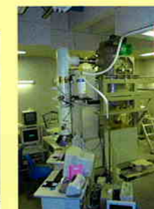
Atom-discriminating electron microscope
