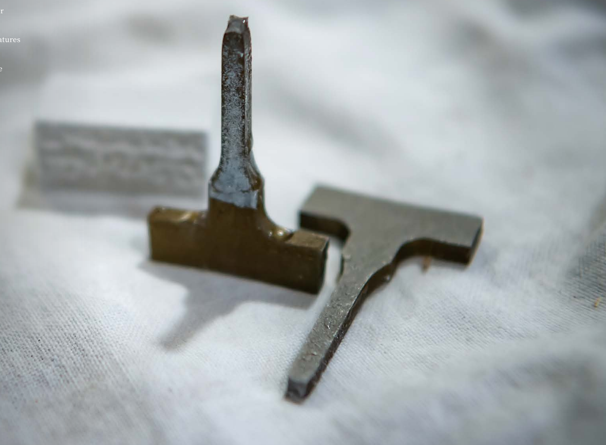
Metallic specimen fractured via slow strain rate tensile test—a test specially designed to study the impact of hydrogen exposure on metallic materials under cryogenic conditions (see p. 15 for details).
