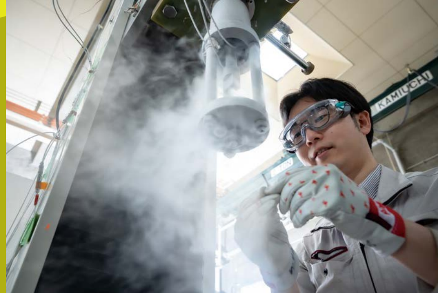
Slow strain rate tensile test being conducted at the temperature of liquid nitrogen (see also the photo of a metallic specimen fractured via this test on p. 2)
