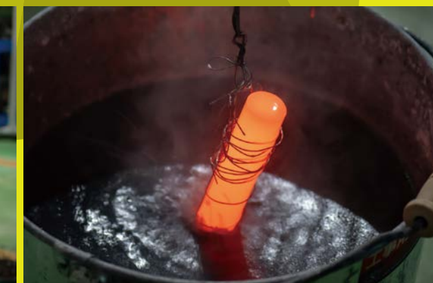
A steel specimen is immersed in a salt bath (i.e., high-temperature molten salt), which is a basic heat treatment for controlling steel microstructure. The physical properties of steel can vary widely depending on the treatment temperatures and cooling rates.
