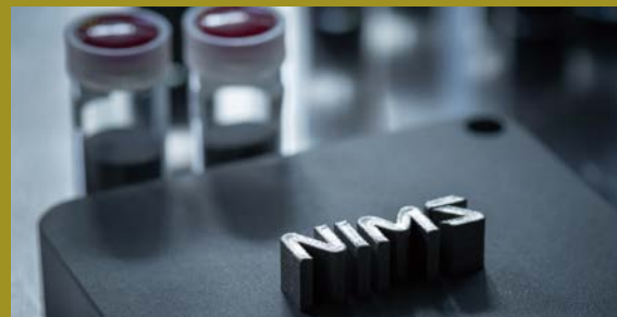
Three-dimensional object created by depositing a material layer by layer using laser powder bed fusion technology
