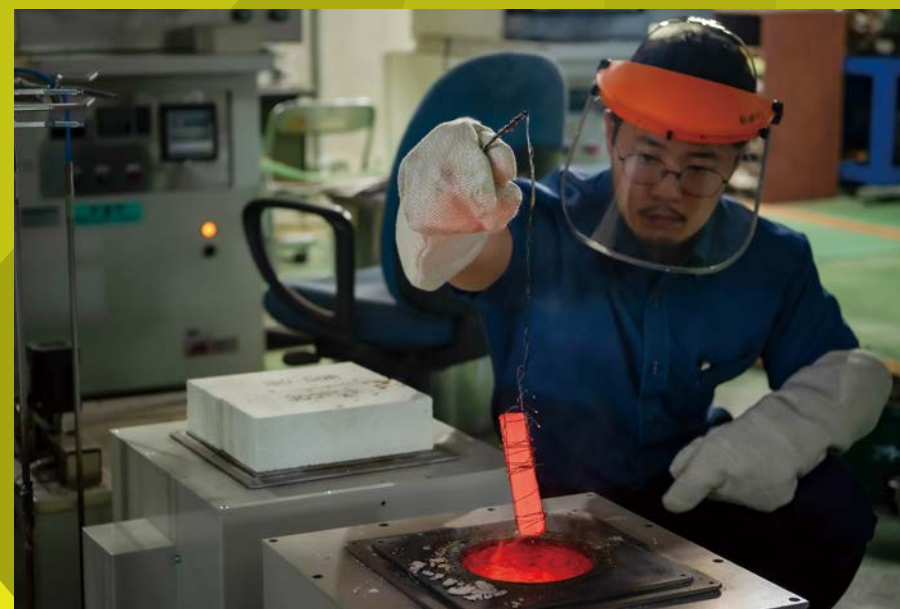
A steel specimen is immersed in a salt bath (i.e., high-temperature molten salt), which is a basic heat treatment for controlling steel microstructure. The physical properties of steel can vary widely depending on the treatment temperatures and cooling rates.
