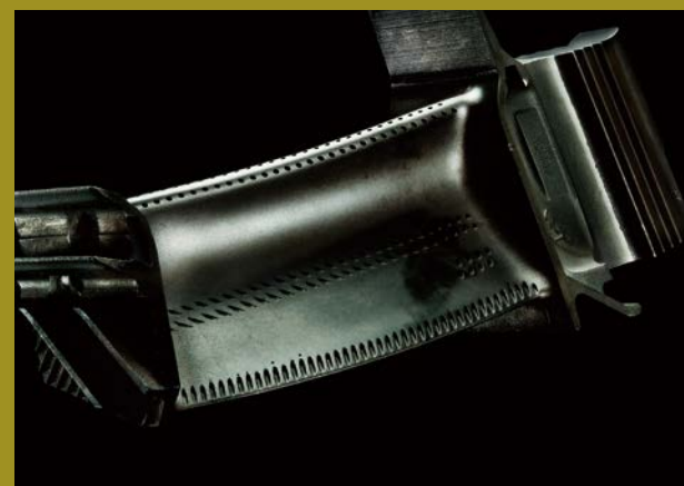
Aircraft engine turbine blade made of the heat-resistant nickel-based superalloy developed by NIMS (photo: Naohiro Tsukada)
